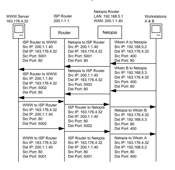
As you can see, when Workstation A and Workstation B transmit an IP packet to the WWW server on the Internet, they have unique source IP addresses on the LAN interface but potentially the same source ports, which in this case is 400. When the Netopia R5000 Series Router receives these packets, the source IP addresses are substituted with the single globally unique IP address that was acquired on the WAN interface, which is 200.1.1.40.
